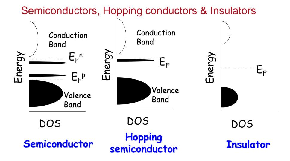
In a semiconductor/insulator there is an energy gap between the filled bands and the empty bands. The distinction between a semiconductor and an insulator is artificial, but as the gap becomes large the material usually becomes a poor conductor of electricity. A hopping semiconductor results when the Fermi level falls within narrow band, W<k<sub>B</sub>T, polarons, impurities, disorder.
