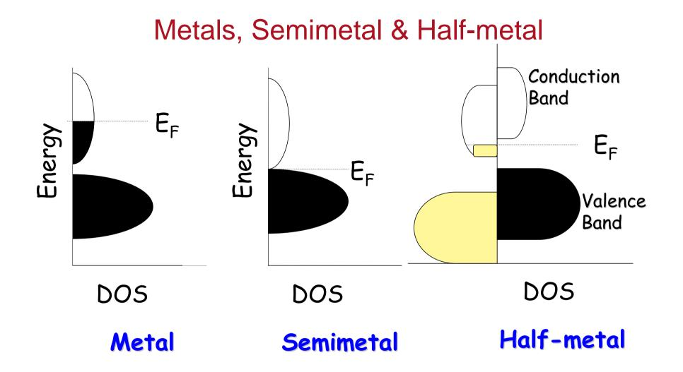
In a metal the Fermi level cuts through a band to produce a partially filled band. A semimetal results when the band gap goes to zero. A half metal results when there is only one spin (up or down) of charge carriers.
